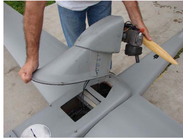
INTEGRAL ENGINE-PYLON-FUEL TANK : TWO PINS /ONE CONNECTOR
